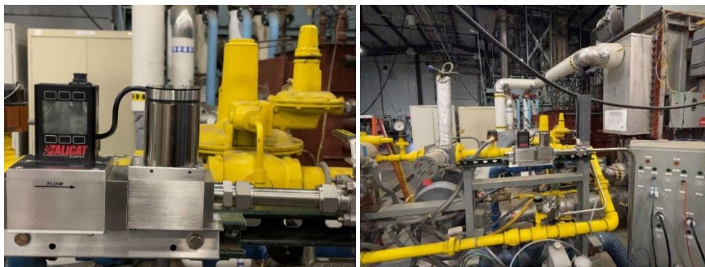
Figure 6. Flow meter mounted in fuel-air skid
