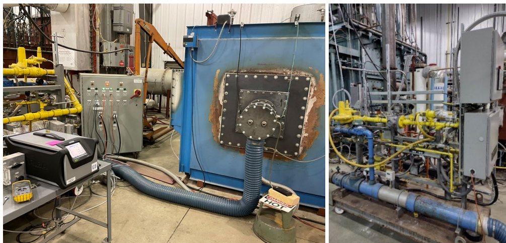
Figure 5. Test setup showing burner mounted on the furnace (left) and air-fuel skid (right)
